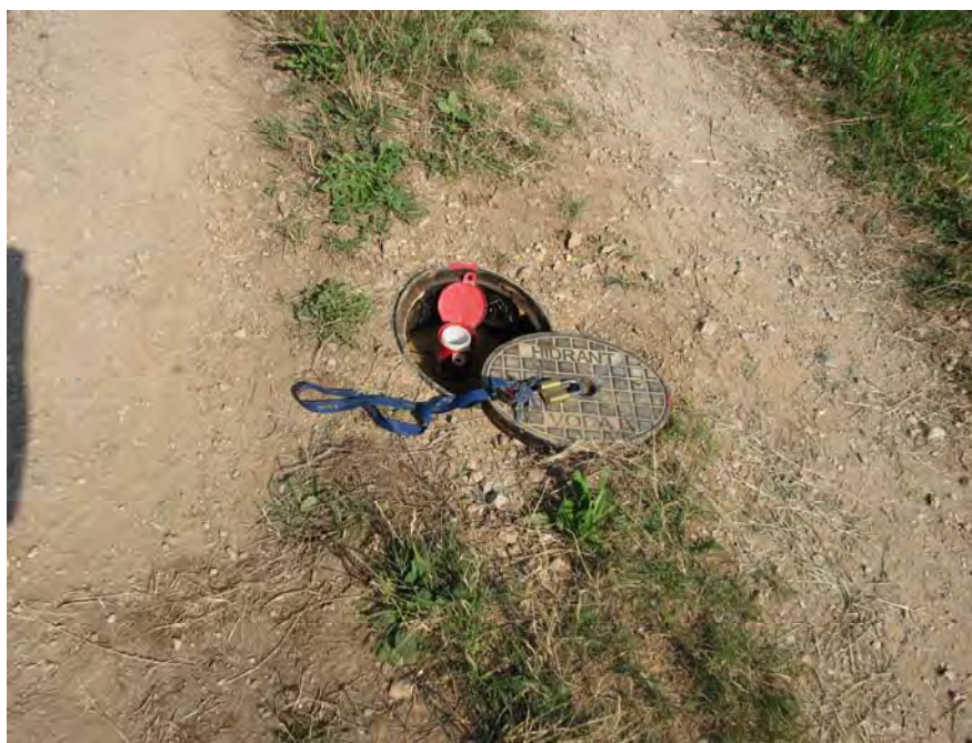
Figure 5: Observation well installed on the field path with street cap and piesometer cap with padlock.
