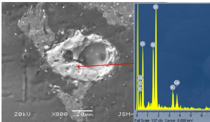
Figure 3. Micrograph of the amorphous grain in the sample A2, with the EDS analysis.
