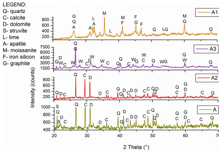
Figure 2. XRD patterns of samples A, A2, A3 and A1.
