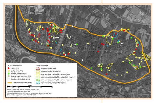
There is reasonable suspicion that additional quantities of past waste are deposited under the surface on 359 dumping sites (24.8 %). Unfortunately, this suspicion applies especially at the major dumping sites where we registered 87,009 m<sup>3</sup> or 41.5 % of the total quantity of waste. More than two thirds (67.5 %) of illegal dumping sites are located less than five meters from access roads.
