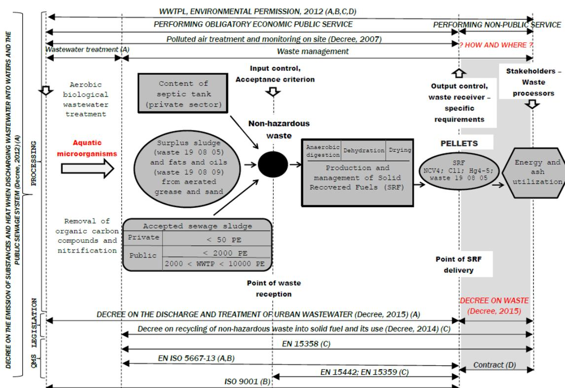
Figure 1: The management system for municipal wastewater treatment and SRF production at WWTP
