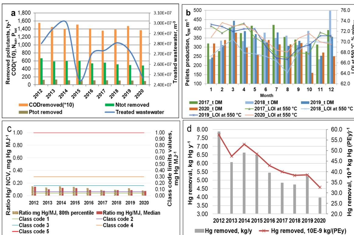
Figure 2: Dynamics of WWTP: a) outflow, COD, nitrogen and phosphorus removal rate per year, b) pellet's production and LOI at 550 °C, c) SRF classification (ratio Hg/NCV of 10 monthly subsamples), and d) annual removal rate of Hg
