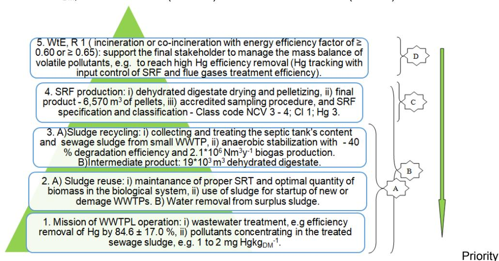
Figure 3: Integrated implementation of wastewater treatment and WtE procedures in terms of waste hierarchy (WFD, 2008), reduction of carbon footprint, and prevention of Hg circulation in the environment
