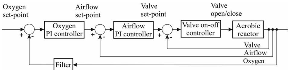
**Figure 6** | Control scheme of the oxygen control.
