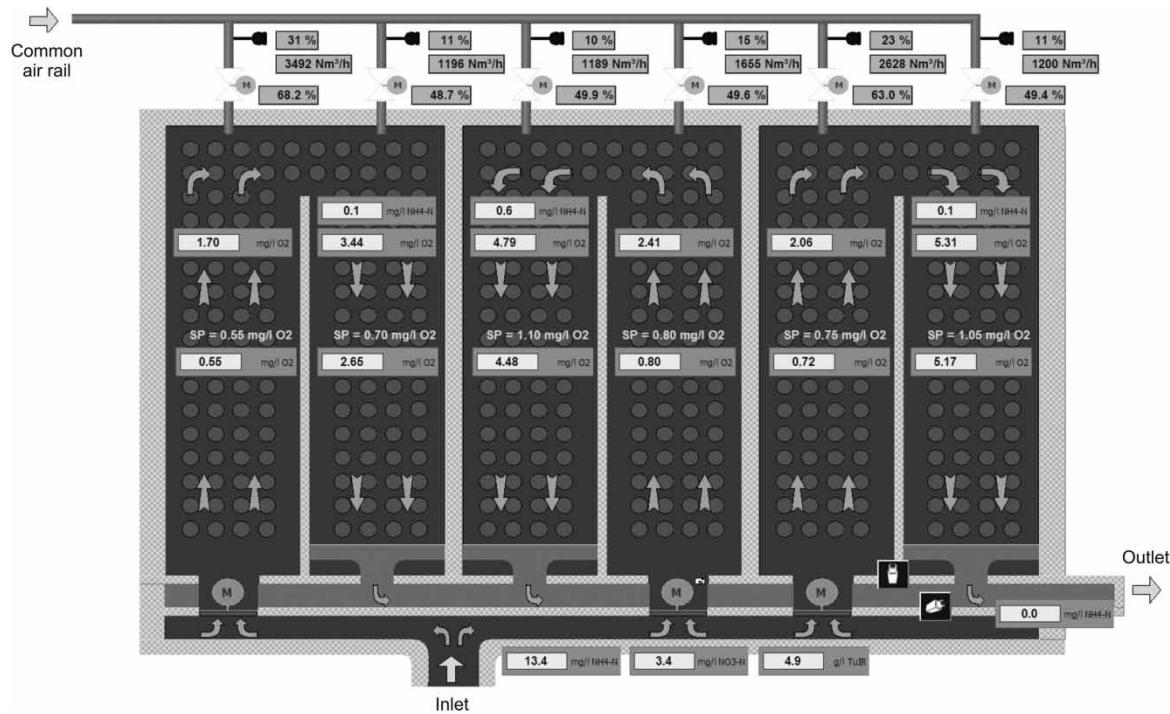
**Figure 1** | Scheme of the aerobic reactors and the common air rail at the Ljubljana WWTP.
