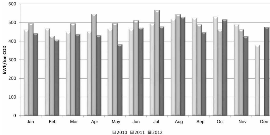
Figure 8 | Monthly electricity consumption for aeration at the Ljubljana WWTP in 2010, 2011 and 2012.
