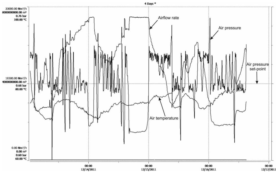
**Figure 2** | Results of the initial air pressure controller for 4 days of operation. Signals shown: air pressure, airflow rate and air temperature in the common air rail.
