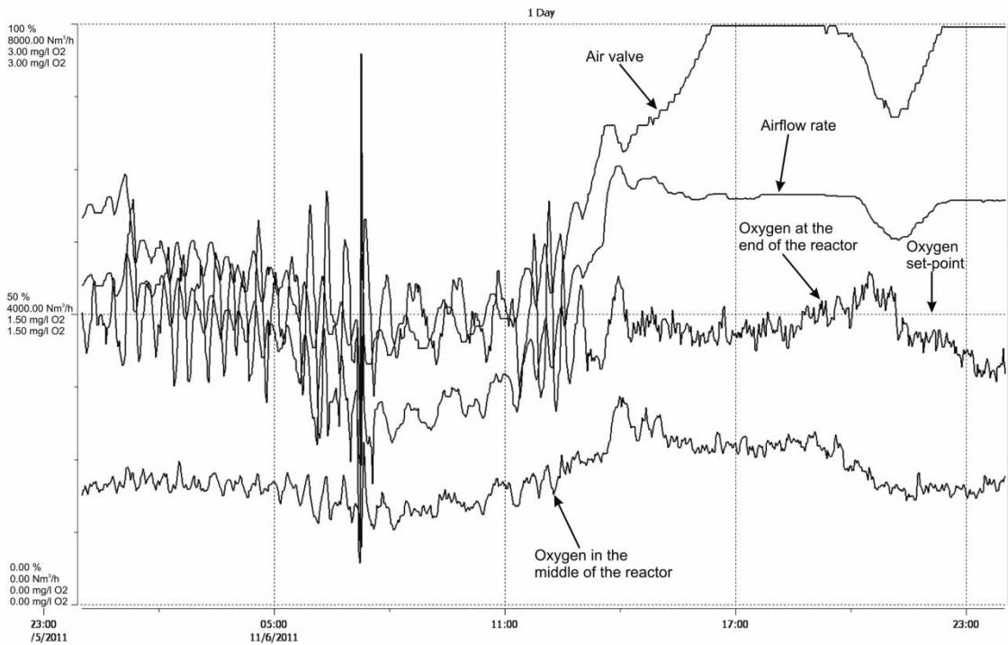
**Figure 5** | Results of the initial oxygen controller in the fourth reactor (the second inlet reactor) for 1 day of operation. Signals shown: oxygen concentrations at two locations, air valve value and airflow rate.
