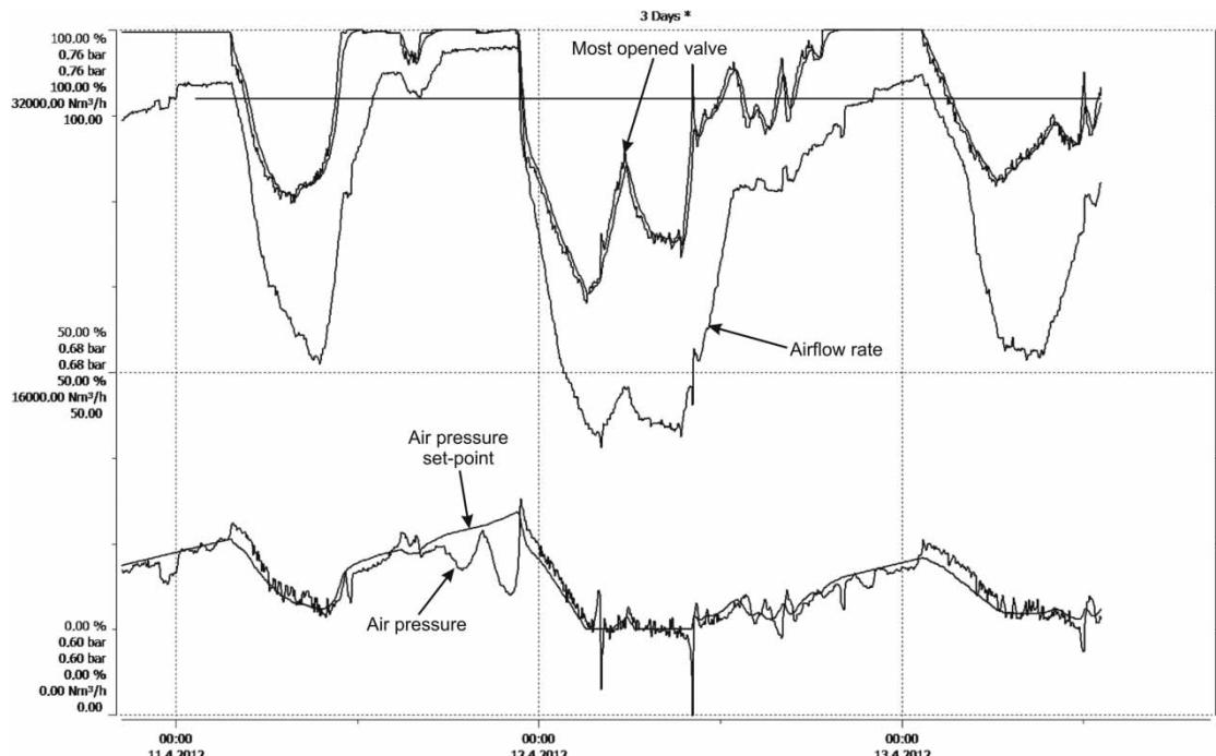
**Figure 4** | Results of the air pressure set-point controller for 3 days of operation. Signals shown: air pressure and airflow rate in the common air rail and the most opened air valve (non-filtered and filtered value).
