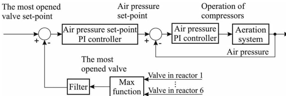
Figure 3 | Control scheme of the air pressure control.
