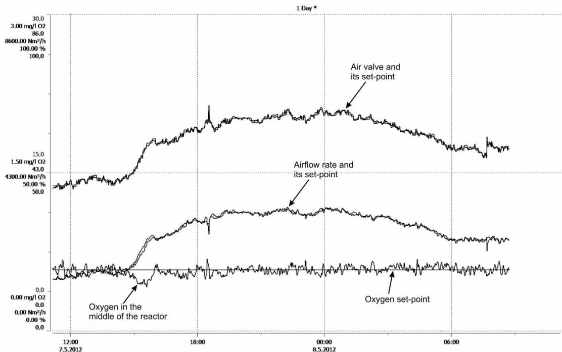
**Figure 7** | Results of the improved oxygen controller in the fourth reactor (the second inlet reactor) for 1 day of operation. Signals shown: oxygen concentration, air valve value and airflow rate.
