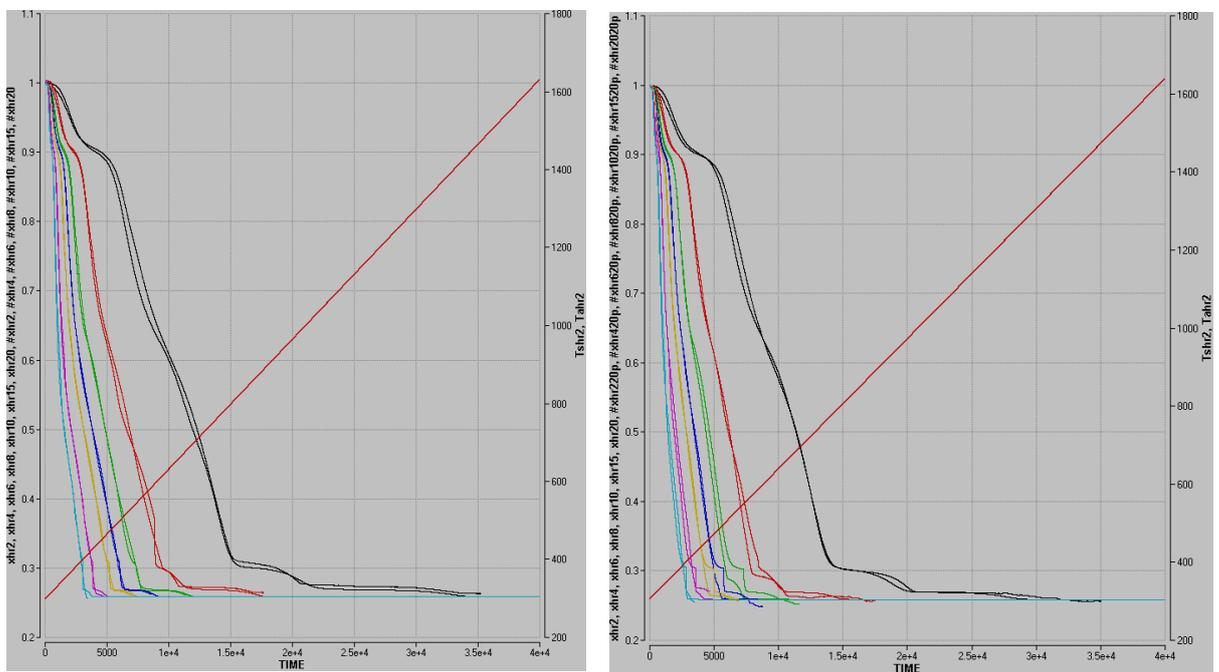
Graph 3: Measured and predicted weight loss using 10% (left) and 20% (right) oxygen in carrier gas phase.
