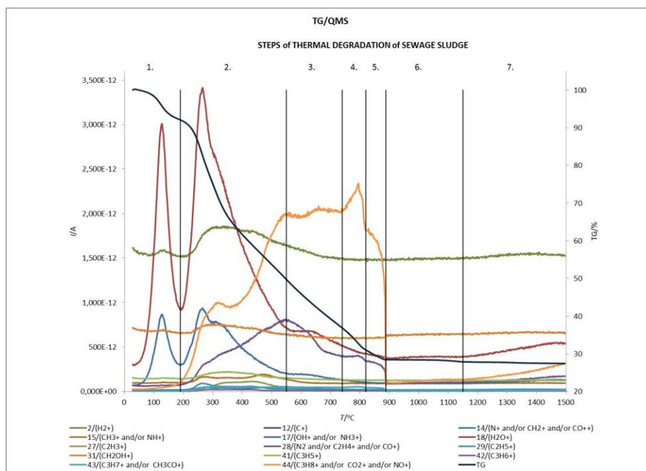
Graph 1: Combustion fingerprint of sewage sludge at oxidative atmosphere in temperature range from 28 °C to 1500 °C.
