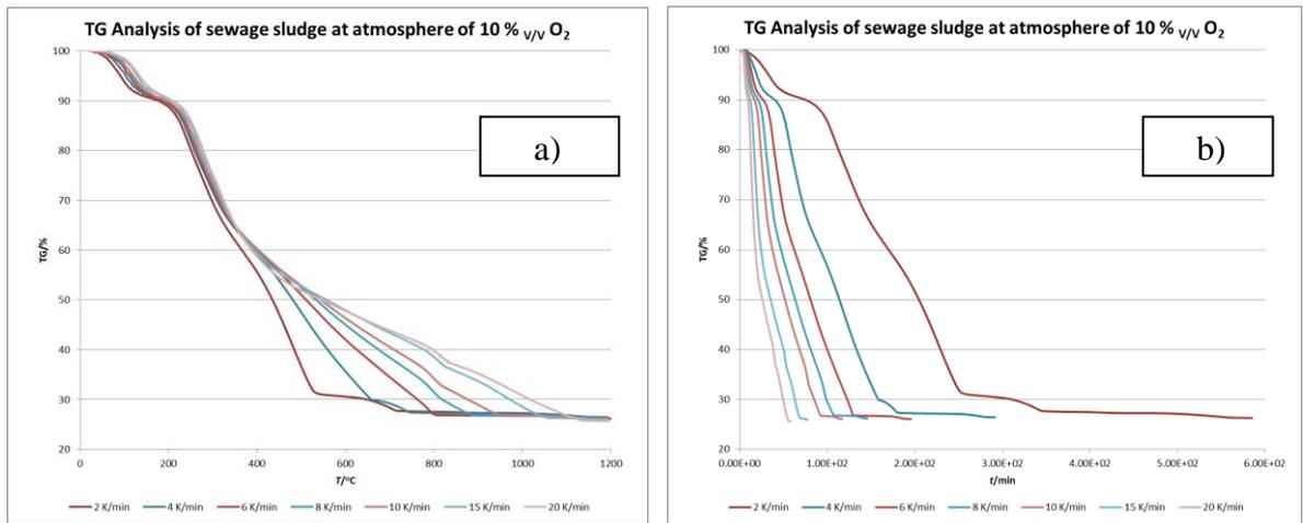
Graph 2: a) The dependance of mass loss according to the temperature and b) according to the time of combustion process.
